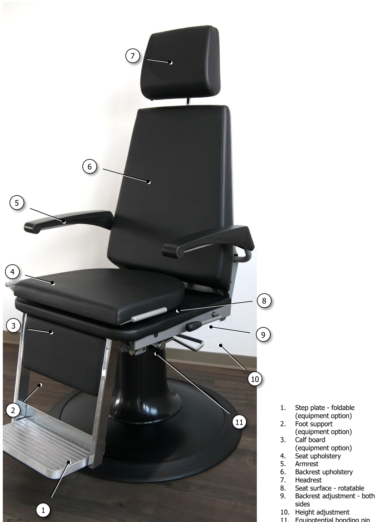
Fig. 6 Structure of the chair - hydraulic height / manual backrest adjustment and rotatable seat surface
